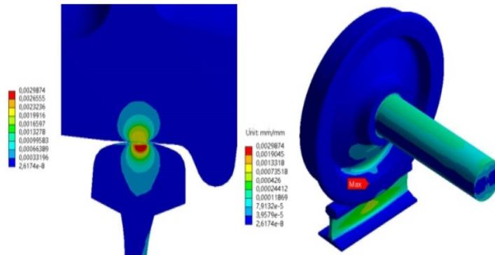
Fig. 11 – Distribution of elastic - specific deformations, *global model*.
