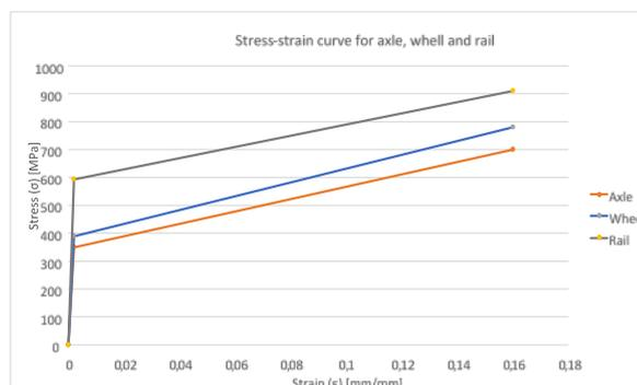
Fig. 2 – The elastic-plastic model adopted for axle, rail and wheel.
