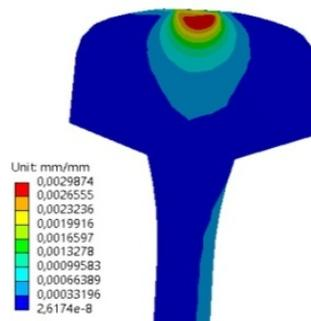
Fig. 12 – Distribution of specific deformations at wheel contact, *rail*.
