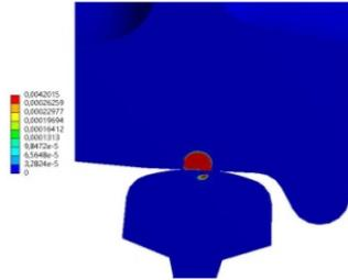
Fig. 14 – Distributions of specific plastic deformations, *global model*.
