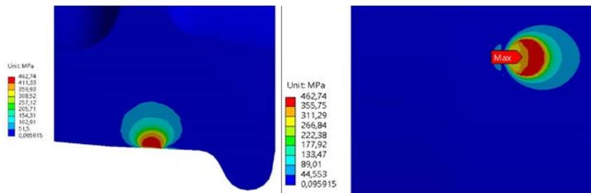
Fig. 8 – Stress distribution at wheel contact, *wheel*.
