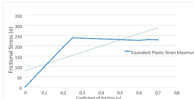
Fig. 10 – Distribution of contact stress function of friction coefficient.
