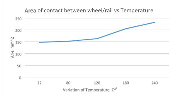
Fig. 18 – Contact area, the elastic - plastic model, vs. temperature.
