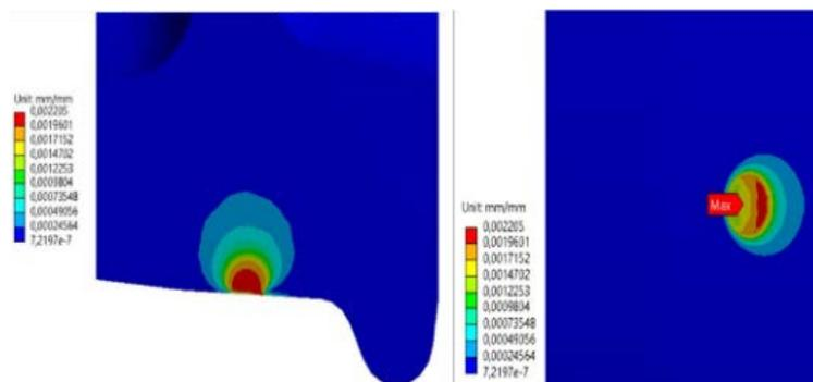
Fig. 13 – Distribution of specific deformations at wheel contact, *wheel*.
