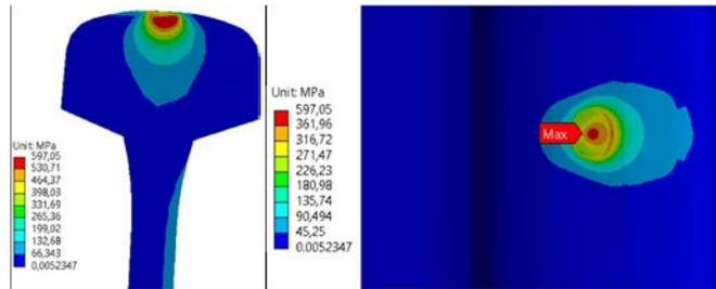
Fig. 9 – Stress distribution at wheel contact, *rail*.
