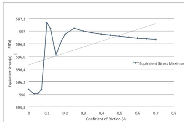
Fig. 6 – Maximum Von-Mises tension versus friction coefficient.
