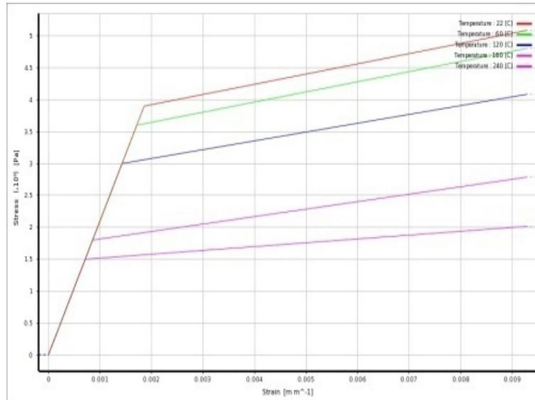
Fig. 3 – The elastic-plastic model of the wheel material vs. temperature.
