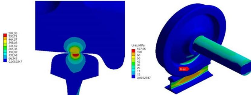
Fig. 7 – Stress distribution at wheel contact, *global model*.
