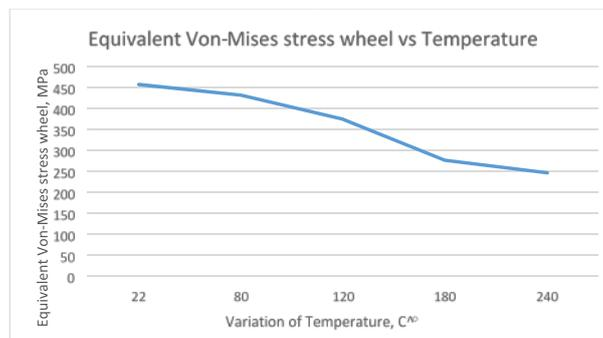
Fig. 19 – Von-Mises stress distribution depending vs. temperature.
